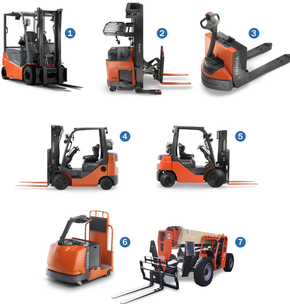
Figure 2.1. Seven classifications of PITs.
