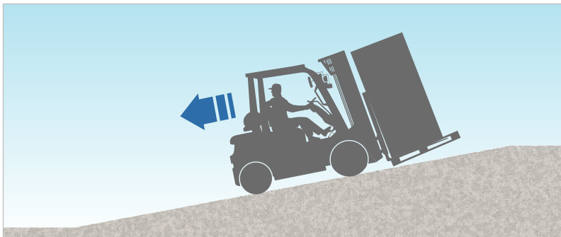
Figure 5.4. When traveling downhill with a load, drive in reverse and look in the direction of travel.
