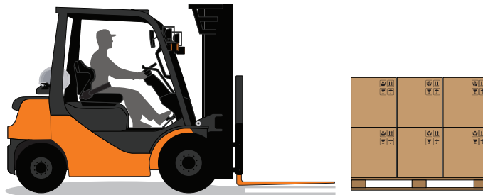
Figure 5.9. Mast is level when approaching a load to lift.
