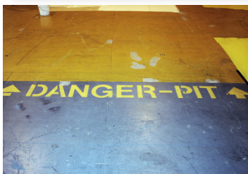
Figure 4.4. Many stages have pits and tanks located under the floor that may not be able to support the weight of a forklift and its load. Contact Backlot Operations or Studio Safety to get authorization to take a forklift onto a stage floor. Check posted signage and the stage itself for weight limits and markings indicating pits and tanks.
