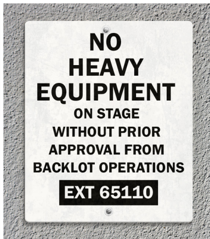
Figure 4.4. Many stages have pits and tanks located under the floor that may not be able to support the weight of a forklift and its load. Contact Backlot Operations or Studio Safety to get authorization to take a forklift onto a stage floor. Check posted signage and the stage itself for weight limits and markings indicating pits and tanks.
