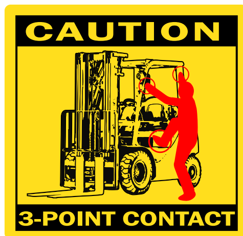
Figure 4.6. Mount and dismount a forklift using three points of contact.
