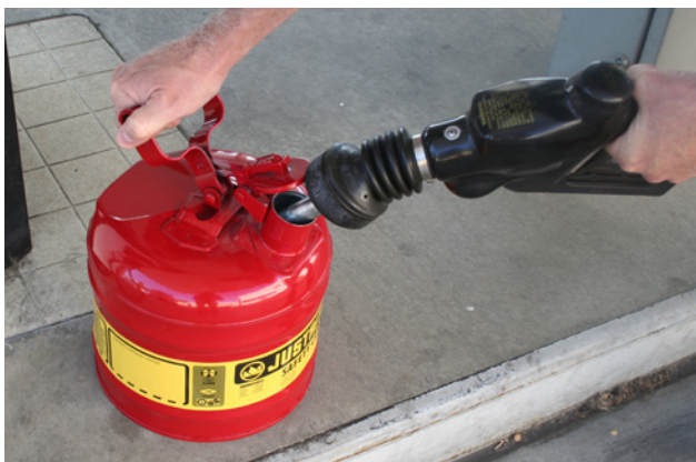
Figure 7.1. Use approved safety cans for fuel and keep the nozzle in contact with the container while filling.
