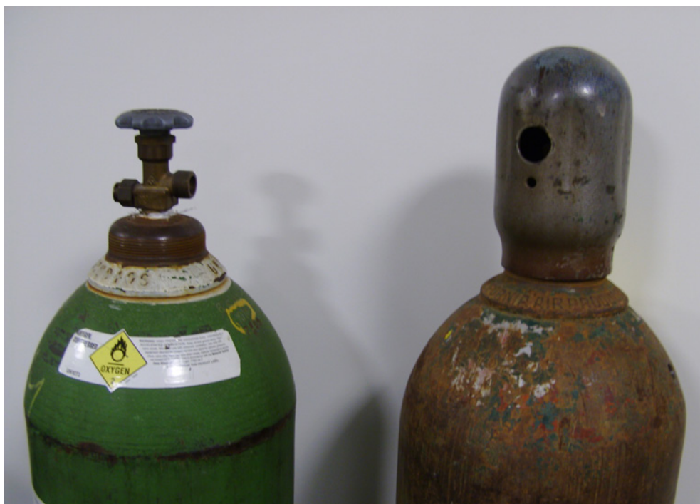
Figure 2.4. Unprotected cylinder (left) and cylinder with valve protection (right).
