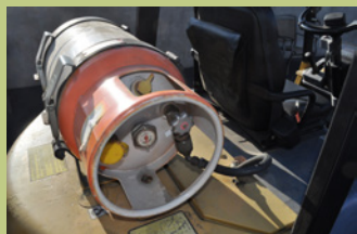
Figure 3.4. Industrial truck LPG fuel tank mounted horizontally.
