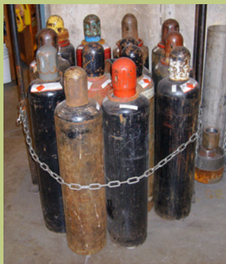
Figure 3.9. Cylinders must be strapped or chained to protect against tipping or movement. Some locations may require two straps or chains, especially in areas prone to earthquakes.
