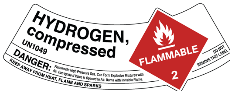
Figure 4.4. All cylinders must be legibly marked with the contents.
