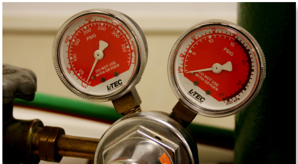
Figure 3.2. Gauges must be correct for the type of gas being used.
