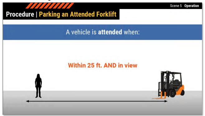
Ok, let's look at a couple of parking procedures. When parking a forklift that will be attended, fully lower the forks or other attachment, put the vehicle in neutral, and set the parking brake. A vehicle is **attended** when the operator is within 25 feet of the forklift, and it remains in view.
