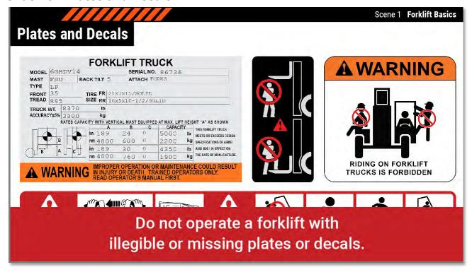
Forklifts have multiple plates and decals that provide important information, instructions, and warnings. Check the operator's manual to see where each data plate and decal is located on the vehicle. Do not operate a forklift with illegible or missing plates or decals.
