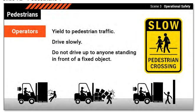
Unfortunately, crushing injuries to workers and other pedestrians from collisions and falling loads is an all-too-common occurrence. It is the operator's responsibility to watch out for and yield to pedestrian traffic, to drive slowly so that there is no need to stop abruptly, and to never drive a forklift up to anyone standing in front of a fixed object.
