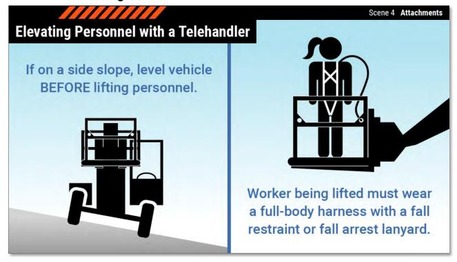
When using a telehandler to elevate workers, ensure the outriggers are placed on a solid surface. If operating on a side slope, level the vehicle before lifting personnel. Each worker being lifted must wear the required PFPE—a full-body harness with a fall restraint or fall arrest lanyard of the appropriate length, connected to an authorized anchor point.
