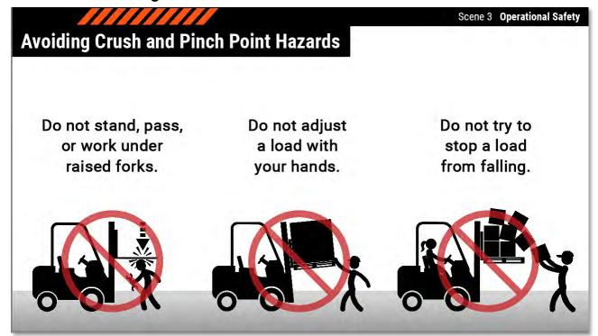
Do not stand, pass, or work under raised forks. Although unlikely, in the event that the hydraulics fail, even empty forks can crash down hard. Do not adjust a load with your hands or try to stop a load from falling.
