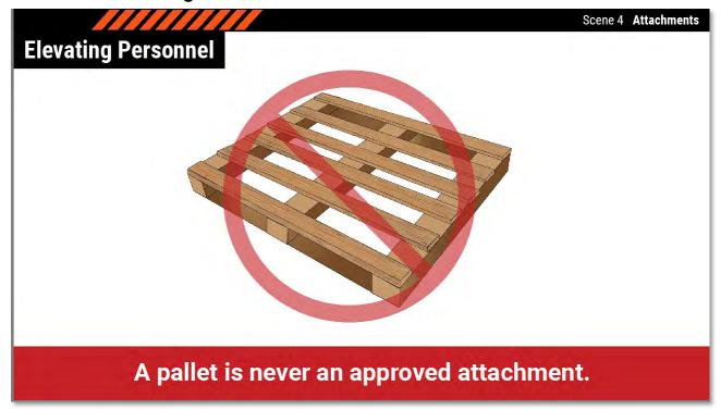
Keep in mind that a pallet is not an approved attachment and should never be used to elevate workers.
