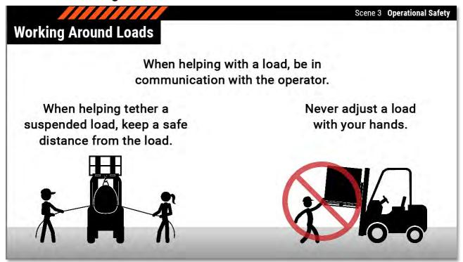
When helping with a load, be in communication with the operator. When helping tether a suspended load, keep a safe distance from the load. And, never adjust any load with your hands. This can result in crushing injuries.
