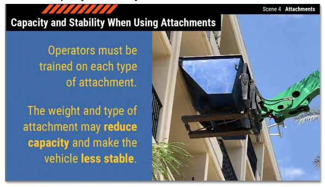
Forklift operators must be trained on how to use each type of attachment. The weight and type of attachment may reduce capacity and make the vehicle less stable, increasing the chance of a tip-over.
