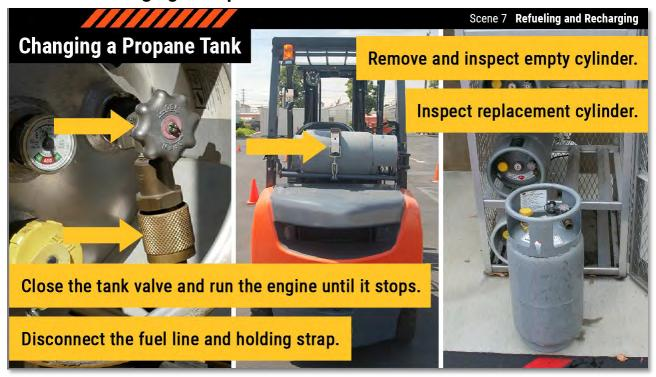
Close the tank valve and run the engine until it stops to ensure that the fuel line is empty. Carefully disconnect the fuel line and holding strap. Remove the empty cylinder and inspect it for damage. Then, inspect the replacement cylinder. Remove any damaged cylinder from service.
