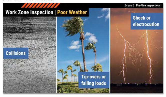
Lastly, is there a possibility of poor weather? Operating a forklift when it's raining, windy, or there's a chance of lightning can put you or others at risk of being injured by collisions, tip-overs, falling loads, shock, or electrocution.
