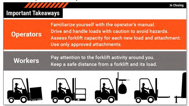
If you are an operator, familiarize yourself with the operator's manual before operating any forklift. Drive and handle loads with caution to avoid common hazards like collisions, tip-overs, and falling loads. Assess forklift capacity for each new load and attachment. And, use only approved attachments. If you are a worker, pay attention to the forklift activity around you and keep a safe distance from a forklift and its load.
