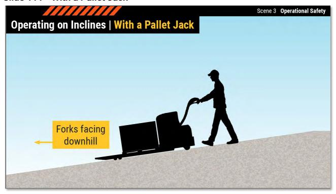
To keep a motorized or hand pallet jack from rolling into you, keep the forks pointed downhill regardless of whether there is a load on the forks or not.
