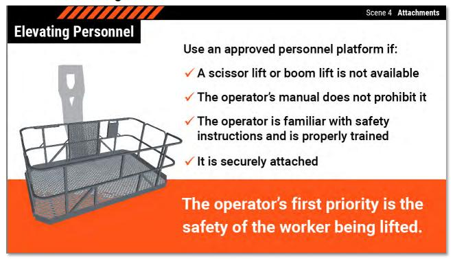
A personnel platform approved by the manufacturer can be used to lift workers to work positions if there is no other practical option available, such as a scissor lift or boom lift, the operator's manual does not prohibit it, the operator is familiar with safety instructions and is properly trained in its use, and it is securely attached. When elevating workers, the forklift operator's first priority is the safety of the worker being lifted.
