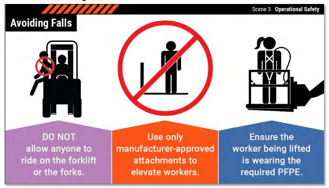
To keep your coworkers safe, DO NOT allow anyone to ride on the forklift or the forks, use only manufacturerapproved attachments to elevate workers to work positions, and ensure that any worker who is being lifted is wearing the required personal fall protection equipment (abbreviated as PFPE). We'll talk more about elevating workers in the next scene.
