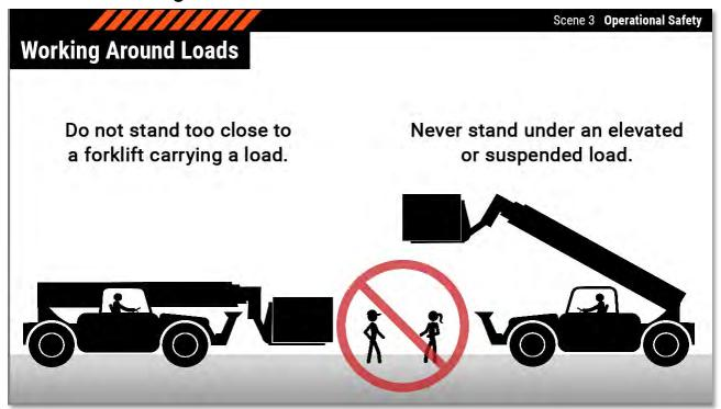
Workers: Do not stand too close to a forklift carrying a load, and never stand under an elevated or a suspended load.
