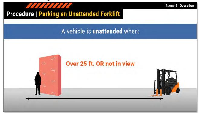
A vehicle is **unattended** when the operator is over 25 feet from the forklift, or it is not in their view.
