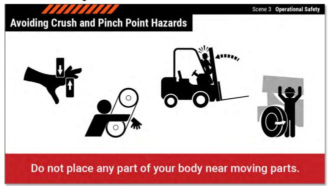
Crush and pinch point hazards are dangerous areas on or around a forklift where one's body or a body part could get caught, resulting in potentially serious injuries. Do not place any part of your body through the mast or mast chains, between the mast and cab, between a wheel and the forklift, or near any other moving parts of the vehicle. Wind has the potential to blow clothing and long hair into moving parts of the mast. Do not wear loose-fitting clothing or scarves and tie back long hair.
