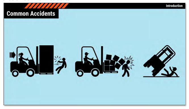
The most common forklift accidents are collisions, falling loads, and tip-overs, all of which can result in injuries to a pedestrian, a worker, or the forklift operator, as well as damage to the load, the vehicle, or other property.
