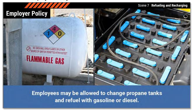
Depending on employer policy, you may be allowed to change propane tanks and refuel forklifts that use gasoline or diesel fuel. However, only qualified and authorized persons may refill propane tanks and change and recharge batteries.
