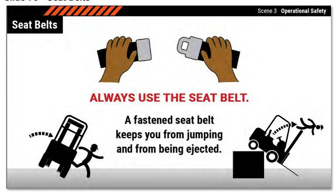
Let's start with one of the most important and basic safety requirements--wearing the seat belt. Always wear your seat belt when operating a forklift, even if the ride is short or you get on and off the vehicle frequently. During a tip-over, a fastened seat belt keeps you from jumping from the vehicle and being crushed. A seat belt also keeps you from being ejected during a collision.
