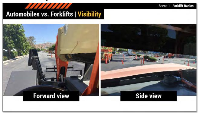
Here, you can see the forward and side views from the driver's seat of a telehandler. Even unloaded, the boom, outriggers, and engine compartment reduce visibility.
