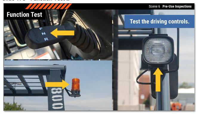
Then, test the driving controls: the steering and horn, the brakes and the inch control (if the vehicle is equipped with it), forward and reverse directional control, the lights, and the back-up alarm.
