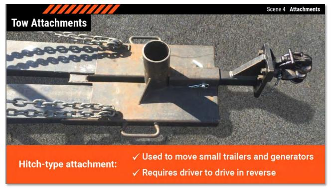
A commonly used attachment in our industry is the hitch-type attachment used to move small trailers and generators into place. These towing attachments require the driver to drive in reverse, looking in the direction of travel.
