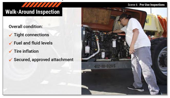
The walk-around inspection requires you to verify the overall good condition of the vehicle. Check for tight connections, proper fuel and fluid levels, proper tire inflation, and that the forks or the approved attachment is properly secured.
