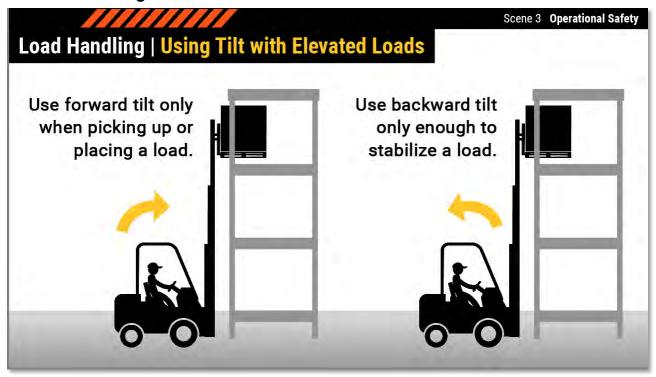
While backward tilt is recommended for stability when transporting a load, using tilt when a load is elevated can result in a falling load or a tip-over. When a load is elevated, use forward tilt only when picking up or placing the load, and use backward tilt only enough to stabilize the load. Do not let anyone stand under or near an elevated load.
