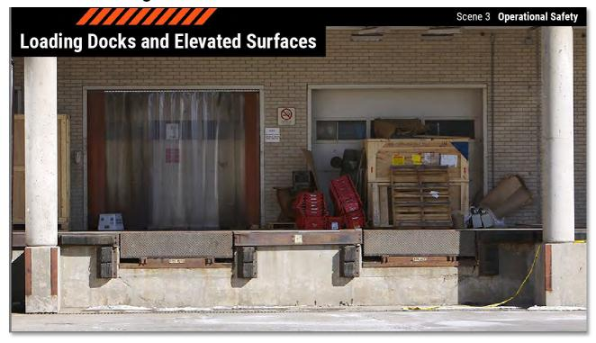
When operating on a loading dock or another elevated driving surface, a major safety issue is driving off the edge. This type of tip-over can cause serious crushing injuries. Maintain a distance of at least one tire width from any edge. And, it is especially important on loading docks to be careful of the rear swing of the vehicle when turning.
