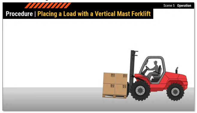
Now, we'll place a load using a vertical mast forklift. Square the forklift to the placement area. Level the mast so that there is no tilt. Position the load to the necessary height, and drive forward slowly and carefully. Lower the load until it is securely placed. Continue to lower the forks until the load is disengaged. Back away slowly, looking in the direction of travel, and be careful that the forks do not hit the load or pallet. Adjust the fork height for safe travel.
