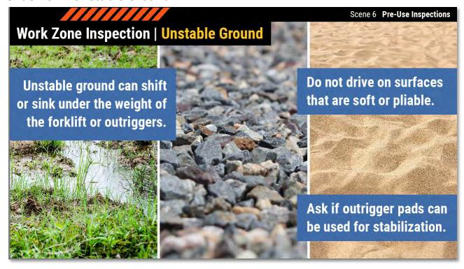
When working on location or on a backlot, there may be unstable ground such as mud, grass, gravel, and sand. These types of surfaces can shift or sink under the weight of the forklift or the outriggers, leading to falling loads or tip-overs. Check for surfaces that are soft or pliable, and ask your safety representative if outrigger pads can be used to stabilize a work surface.
