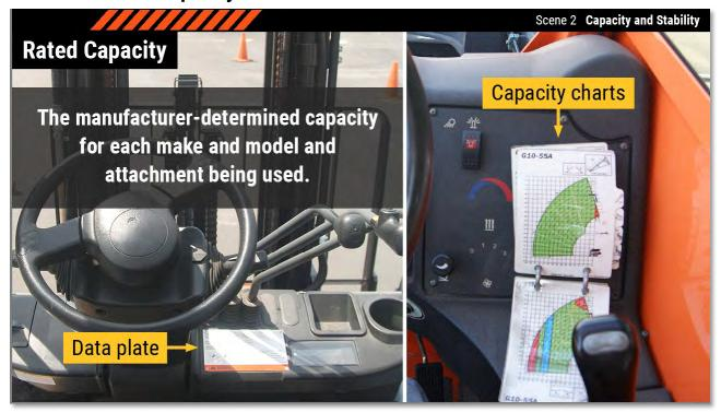
Now, let's talk about **rated capacity**. Rated capacity is the manufacturer-determined capacity for each make and model of forklift and the attachment being used. On a vertical mast forklift, the rated capacity is shown on the data plate. On a telehandler, it's on capacity charts.
