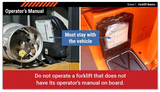
Each forklift has its own operator's manual, which must stay with the vehicle. Forklift operators should use it to familiarize themselves with that make and model's operation, safety, and emergency instructions. Do not operate a forklift that does not have its operator's manual on board. If the manual is missing, contact your transportation department or safety representative.
