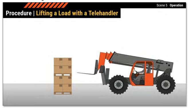
Lifting a load with a telehandler is a bit different than using a vertical mast forklift. First, you'll level the carriage, not the mast. Next, insert the forks under the load by driving forward or extending the boom, depending on where the load is placed. Then, lift the load and tilt it back for added stability. Finally, retract the boom fully and position it for safe travel.
