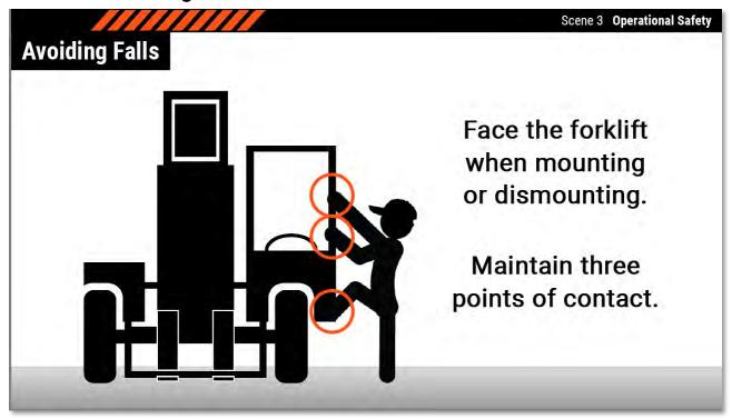
A fall is another serious hazard for forklift operators and other workers. To avoid being injured when mounting or dismounting a forklift, face the vehicle and always maintain three points of contact.
