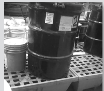
Figure 7.3. Containers of hazardous waste must be labeled.
