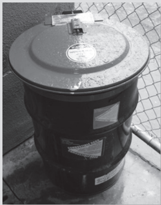
Figure 6.6. Rags with ignitable solvents should be stored in a vented container, kept separate from other solid waste, and removed at the end of the work day.
