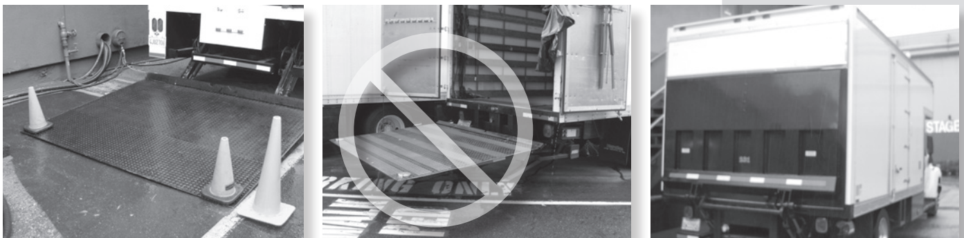
Figure 2.5. Liftgate positioned flat on the ground (left), partially elevated (middle), and stowed (right).
