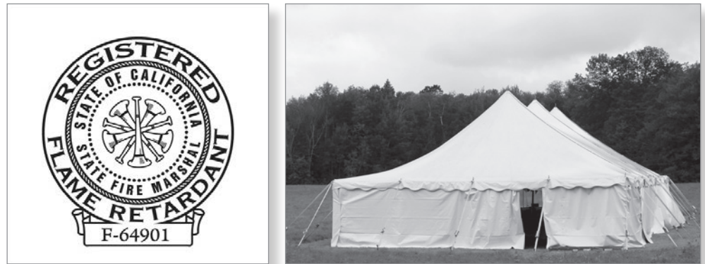
Figure 6.11. Look for this symbol (left) on the tent fabric (right) to confirm that the tent has been treated with an approved flame retardant. A CPAI-84 tag or field test may satisfy this requirement.
