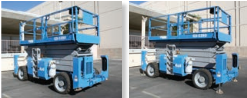
Figure 4.6. This Genie scissor lift is equipped with outriggers. When they are not in use (left), the platform can be raised to 30 ft. When they are extended (right), the platform can be raised to 53 ft.
