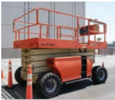
Figure 2.3. Rough terrain scissor lifts are usually engine-powered, and have large, rugged tires. They are better-adapted than an indoor lift for work on uneven surfaces and inclines.
