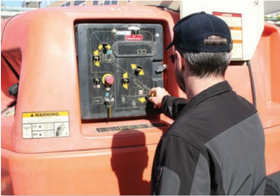
Figure 3.5. Check a lift's functions from the ground controls before operating it from the platform.
