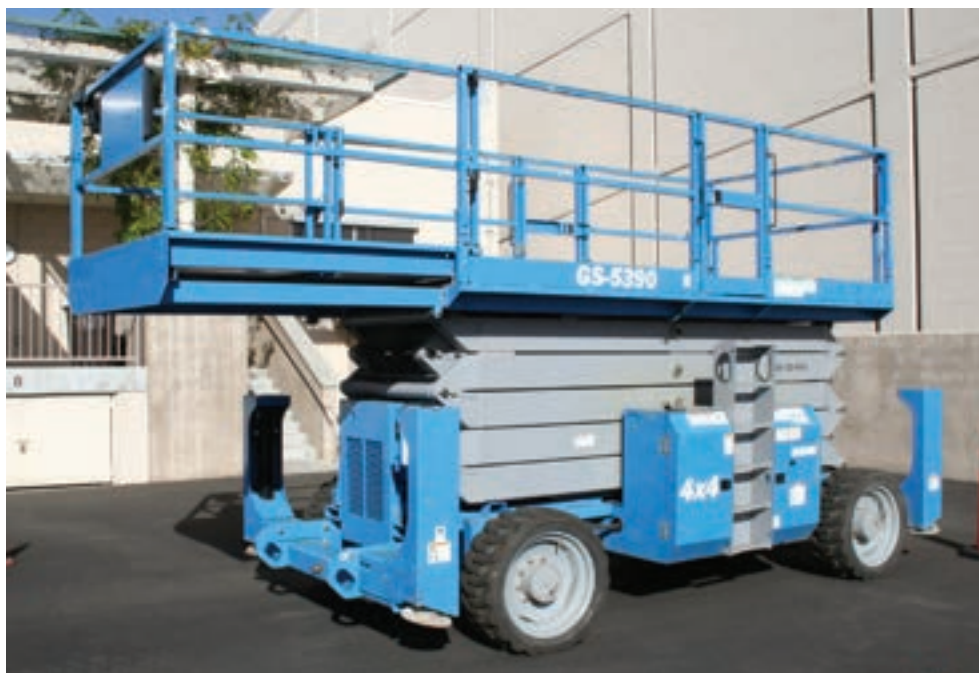
Figure 3.6. Check a scissor lift's platform extension(s) as part of the function check.
