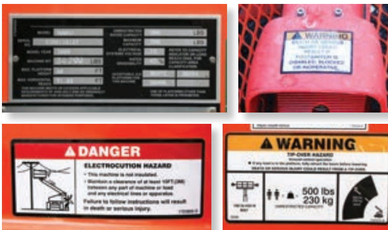
Figure 2.5. Read and understand information plates and warning decals before operating a lift.
