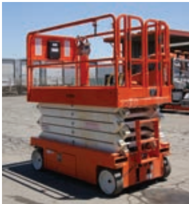
Figure 2.2. Electric scissor lifts operate on rechargeable battery power, which makes them suitable for indoor use. They have small, solid tires which can only be used on smooth surfaces, usually indoors.
