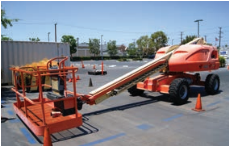
Figure 7.2. Lifts should be in the lowest stowed position when not in use.
