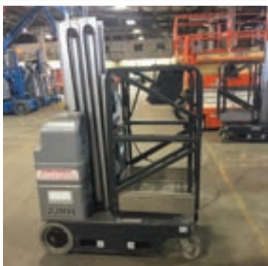
Figure 2.4. Vertical mast lifts are available in “push-around” or electric versions (shown here). If the lift is equipped with outriggers, they must be set before the platform can be elevated.
