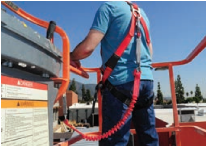
Figure 5.1. PFPE is required in boom lifts (left). Attach lanyards only to authorized anchor points (right). Attach only one lanyard per anchor point.
