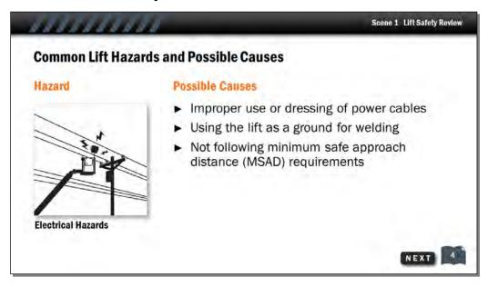
Causes for this include improperly using or dressing power cables, using the lift as a ground for welding, or not following MSAD, or minimum safe approach distance, requirements.
