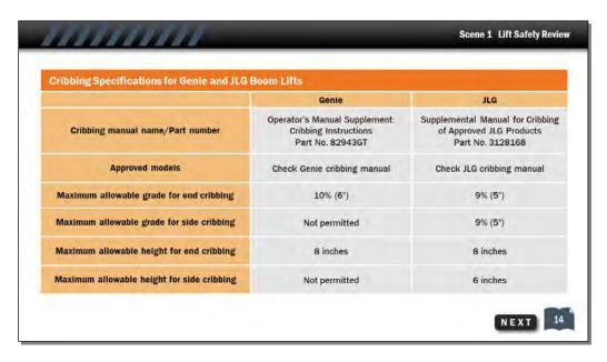
These tables give an overview of the construction requirements for Genie and JLG cribbing. Always follow the manufacturer's specifications and the list of approved models when building or using cribbing.
