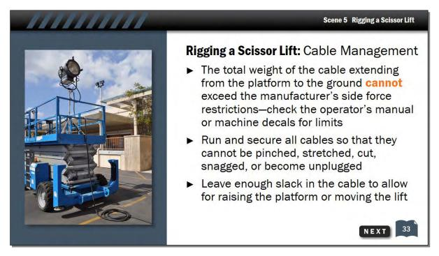
Power cables may extend over the platform of a scissor lift, if these procedures are followed. Most importantly, the total weight of the cable that extends from the platform to the ground CANNOT exceed the manufacturer's side force restrictions, or it could cause a tip-over from a side load. Check the operator's manual for these limits.
