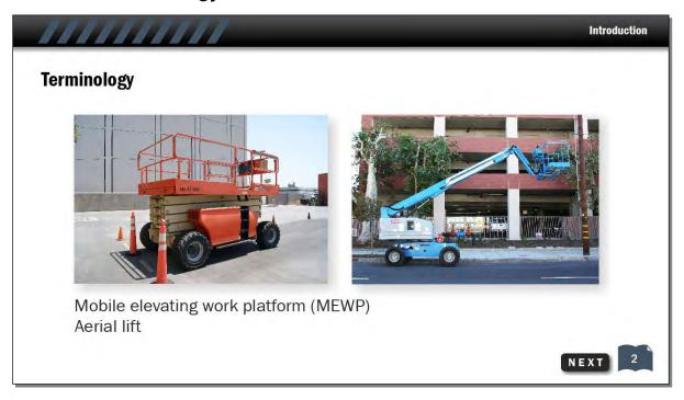
The lifts discussed in this course go by a number of names. In general, they can be called *mobile elevating* work platforms or aerial lifts. In OSHA regulations, a scissor lift is called an *elevating* work platform, and a boom lift is referred to as an aerial device or an extensible boom platform.
