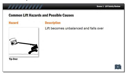
A tip-over is just what it sounds like—the lift becomes unbalanced and tips over, and the operator is injured by being thrown out of the platform or by being crushed by the falling machine.
