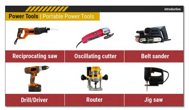
Portable power tools are handheld and can easily be transported to the work site. A few examples of portable power tools are shown here.
