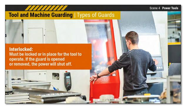
An **interlocked guard** must be locked or in place for the tool to operate. If the guard is opened or removed, the power will shut off.
