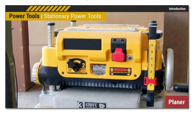
Stationary power tools are mounted to a tabletop or to the floor, such as the tools shown here.
