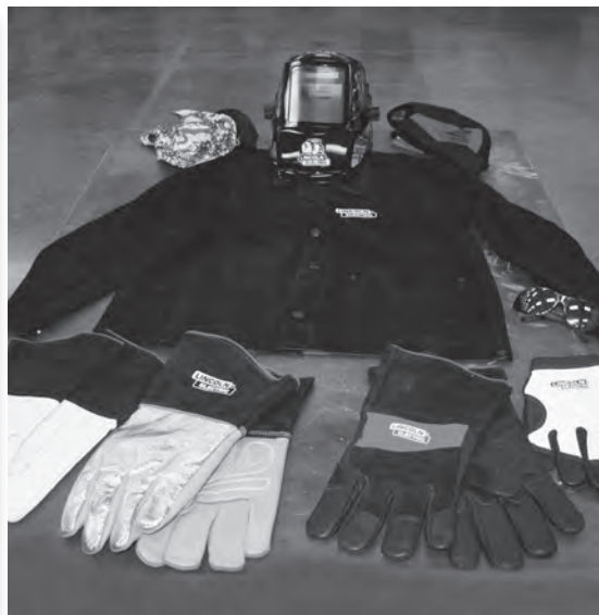
Figure 5.4. Specialized PPE, including helmets, gloves, glasses, and jacket, are used when welding.
