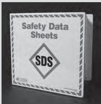
Figure 3.4. If a hazardous chemical is at the work site, a copy of the SDS must be available.
