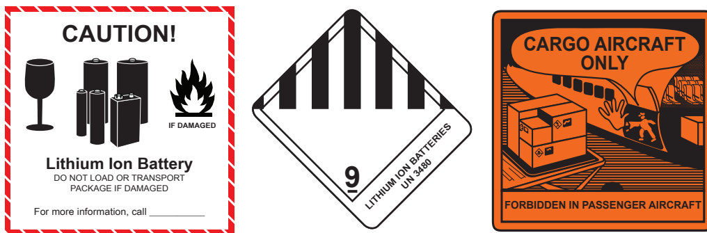
Figure F.1. Required labels for shipping: lithium-ion battery handling label (left), Class 9 Miscellaneous Dangerous Goods label (middle), and cargo aircraft only label (right).
